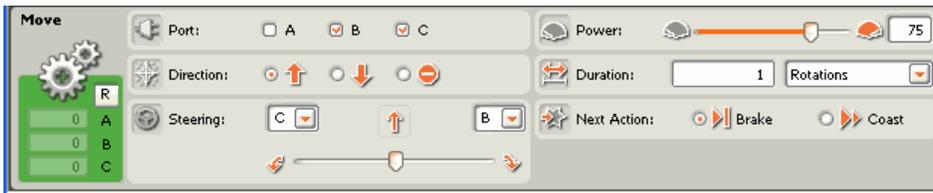
In the port selection, we select where the motors are connected to. In our case, this is port B and C. This is the only thing we have to change here, as we will use the default settings for our first program.
