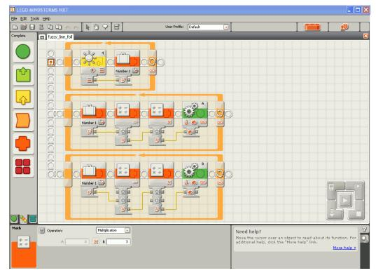
The program consists of three loops that run at the same time. The first loop reads the current reflected light value and stores it in the variable called "Number 1". The second and third loop control the left and right motors.
